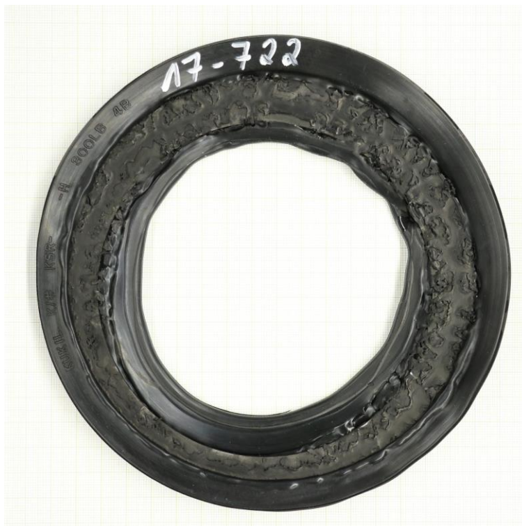
Shell leakage test (T) according MESC SPE 85/300 - 3.3.2
